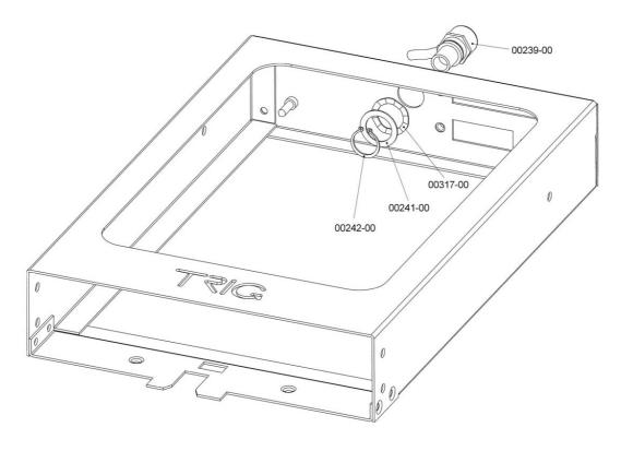
When the BNC is prepared, feed it through the TT31 mounting tray and attach the washer combination in the following order:
