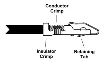
Once crimped, the contacts should be slotted into the rear of the connector shell. Push the contact in until the retaining tab clicks into place. Tug gently to confirm the contact is locked in place.
